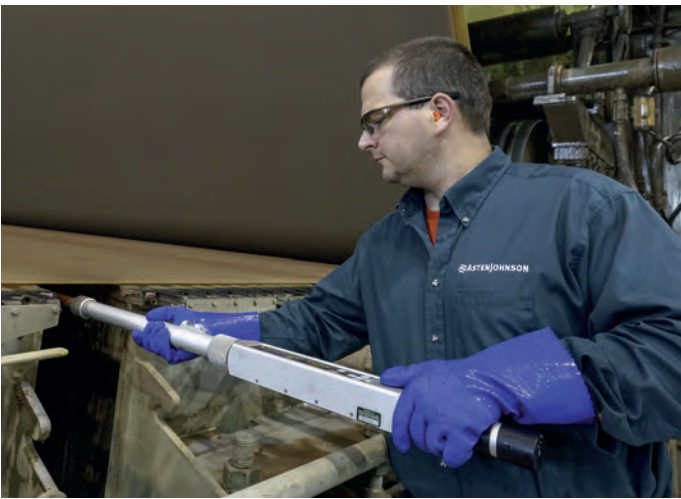
Matt Heiss [AstenJohnson] performing a drainage survey on the former.
